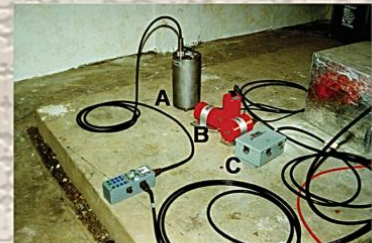
Instrumentation set-up (A- broadband seismometer, B- 3-component short-period seismometers, C- strong-motion seismometer) in seismic stations.
